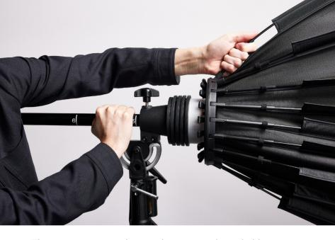
The next step is to make sure that you are always holding on to the back end of the zoom rod with one hand to give you leverage and support when snapping the rods into place.
